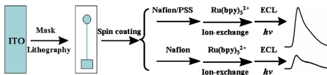
Scheme 1. Schematic illustration of preparation and enhanced ECL intensity of the proposed sensor.
