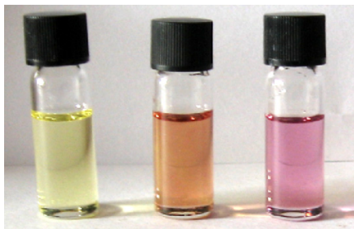
Fig. 2. The color changes of the receptor 1 ( 1 \times 10^{-5} M) with different fluoride concentrations in DMSO. From left to right: (a) only 1; (b) 0.05 equiv. of F^- ; (c) 3 equiv. of F^- .
